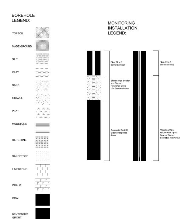
NB Where strata consists of material of more than one soil or rock type the legends are appropriately combined.
